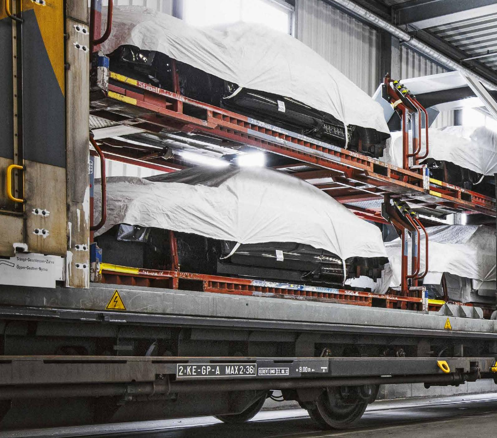
— From loading to unloading, sliding-wall wagons deliver maximum safety for car bodies.
